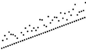
Faulty escapement or damaged pallet stone
