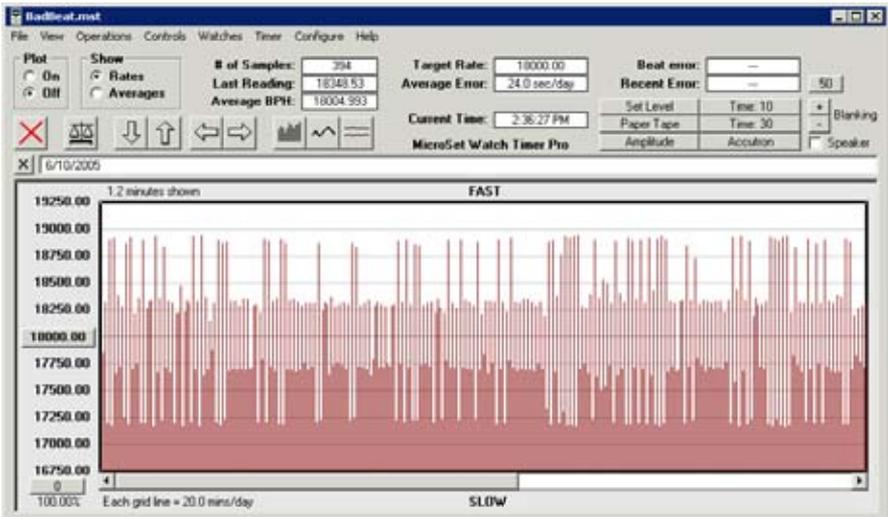
*Inadequate setting of the Level control*
