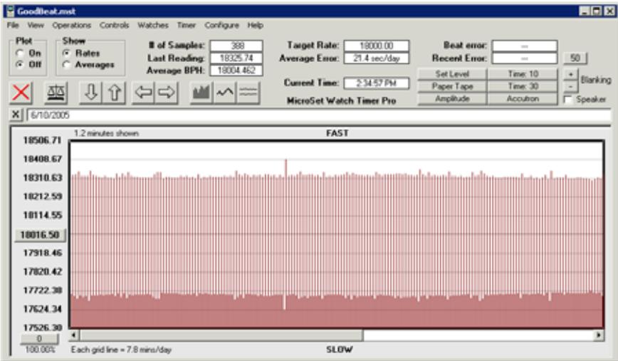
*Consistent readings -- Level control set well*
