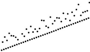
Faulty escapement or damaged pallet stone
