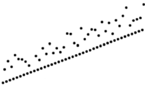
Faulty escapement or damaged pallet stone
