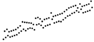
Irregular transmission or dirty escapement
