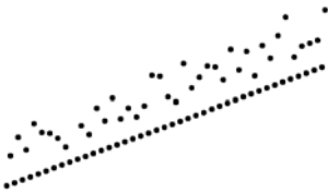
Faulty escapement or damaged pallet stone
